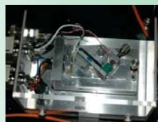
Fig. 1. Schematic of the mechanical setup of the grating-stabilized diode laser system. L. Ricci, et al., Optics Comm. 117, 541 (1995)
